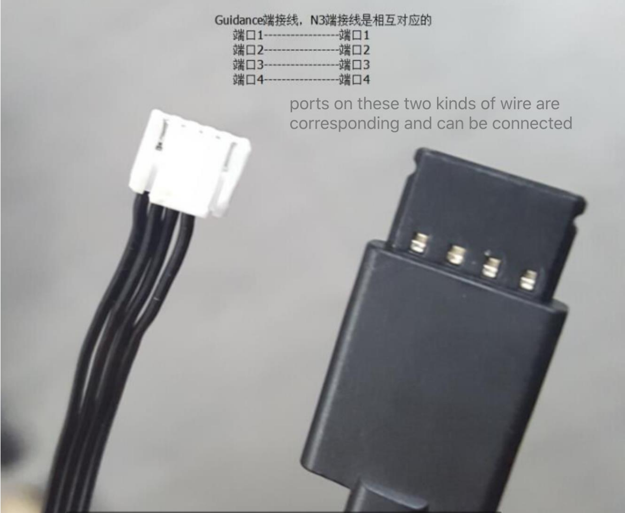
Figure 5. Diagram of connection wires of N3 and Guidance (for the wires on the left, the rightmost port can be left not connected with wire)
