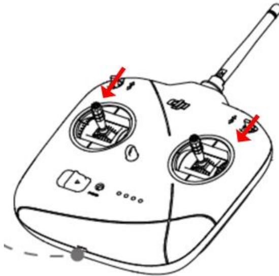
2. Push the left rod to the right and the right to the left. After 2 seconds, the on-board buzzer will make intermittent (1s interval) alerts. Make sure that you perform the third step within 20 seconds, otherwise you'll have to repeat the previous two steps.
