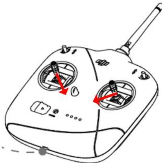
3. Push the left rod to the upper right and the right to the upper left. After 2 seconds, the chassis calibration will be activated and there will be a solid orange light in the ESC. Rotate the right front, left front, left rear as well as the right rear wheels respectively to complete the calibration.
