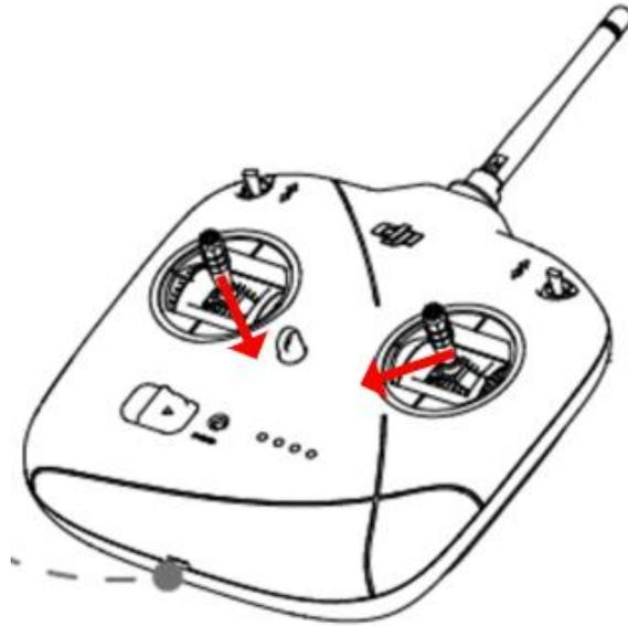
3. Push the left rod to the upper left and the right to the upper right. After 2 seconds, the gimbal calibration will be activated together with continuous high-frequency buzzer alert. The gimbal will begin to move downwards, upwards, leftwards and rightwards respectively. During calibration, do not interfere with the movement of the gimbal.
